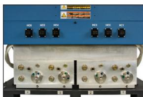
Standard 6 hose/gun connectors, configurable to 8 hose/gun connectors for increased flexibility
