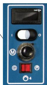
Independent variable-speed pump control provides key-to-line capability
