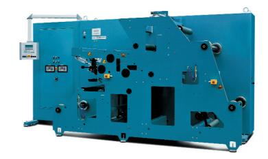
The **CT 5500** series coaters were developed for applications requiring a coating width of 400 to 800 mm (16 to 32 in.). Like the CT 4400 coaters, the CT 5500 coaters incorporate a compact design. The dual-frame roll mounting and distinct, functional design make the CT 5500 Series one of the most flexible units of its kind.
