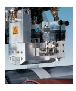
The **Control Coat**<sup>®</sup> system allows hot melt adhesive to be precisely applied without contacting the substrate, providing excellent sharpness in continuous or intermittent applications. This system produces highly dense patterns for maximum bond strength, open patterns when absorbency is important, or extremely thin patterns to eliminate distortion on heat-sensitive substrates.
