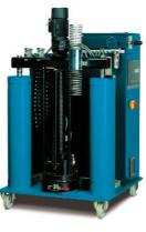
With the **PS** series, Nordson offers customers a bulk melt and metering system which combines highest melt rates up to 1000 kg/hr and big tank capacities (750 kg/ 1650 lb or 1300 kg / 2860 lb) with easy operation – the ideal solution for application with high adhesive consumption. Multiple melt zones provide progressive melting and maintain the integrity of the hot melt adhesives.
