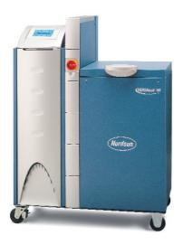
The **VersaBlue®** melters are designed for precise, demanding hot melt adhesive applications. A choice of metering spur-gear pumps with variable-speed AC motors satisfies a wide range of manufacturing requirements. A grid and reservoir tank design reduces adhesive degradation while maximizing adhesive throughput. A VxWorks®-based industrial PC provides full control of the adhesive system via a touch-screen interface.
