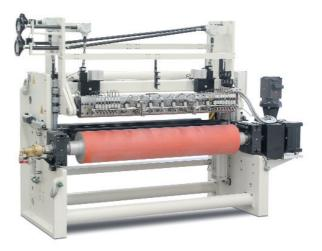
A Nordson specialty, the customized **SB 1000** coating stands are designed for applications with widths up to 4000 mm (157 in.) and can be easily integrated into existing production lines. They can be combined with any coating process, including slot nozzle, screen printing, spray applicator or flexo/gravure roller.
