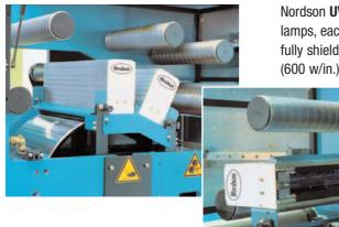
Nordson **UV** drying systems are supplied with medium pressure mercury arc lamps, each fitted in water-cooled, anodized aluminum reflectors and contained in fully shielded and shuttered lamp housings. The nominal lamp rating is 240 w/cm (600 w/in.) depending on the length of the UV lamp. The complete UV drying
