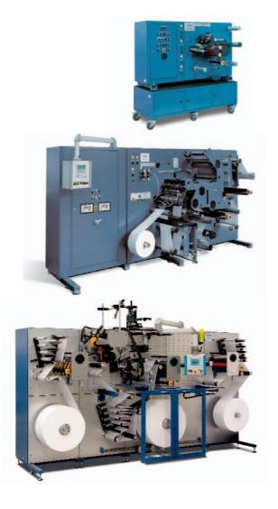
**CL 2000** hot melt lab coaters are widely used in the research and development laboratories of some of the world's most renowned adhesive and raw material manufacturers. Small applications as well as larger volume production trials can be processed at coating widths up to 180 mm (7 in.).
