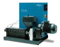
**XP** extruders were developed for processing high-performance, high-viscosity hot melt adhesives and thermoplastics. Extruders of varying sizes with melt rates of 2 to 250 kg/hr (4 to 550 lbs/hr) meet the highest demands regarding precision application by adjusting pressure, torque and motor speed as well as configurations of metering pumps and application heads.
