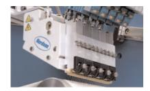
The peak performing **Summit**<sup>™</sup> applicator delivers precise control of adhesive pattern width, fiber size and density for increased bond strength and pattern flexibility. Summit applicators deliver add-on weights as low as 1 g/m<sup>2</sup> at 300 meters per minute. Combinations of full and partial dies enable the customization of applications. The Summit applicator delivers edge control while minimizing overspray.
