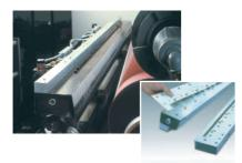
The **BC 31 / BC 35** heads are designed for continuous precision coating. They include 100 percent in-line filtration using a high-volume filter cartridge. The standard coating width is up to 3500 mm (138 in.). Using shim plates in the BC 31, the width and pattern of the adhesive can be modified. The BC 35 coating width can be adjusted up to 350 mm (14 in.) per side within minutes.
