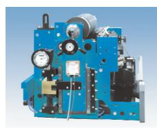
The **Flex-O-Coat**<sup>®</sup> system is suitable for the application of a wide range of patterns. It consists of a special hot melt application roll, a heated transfer roll, and a nip roll. The system combines precise adhesive placement and web handling into a single module that easily retrofits into most roll-fed printing presses and web handling equipment.
