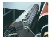
The **BC 40** coating head is designed for continuous applications with standard coating widths up to 3500 mm (138 in.). The "Rotating Bar" produces a streak-free coating. Special Teflon<sup>®\*</sup> profiles can be used to alter the application width.
