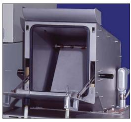
Adhesive-loading elevator protects operator from adhesive backsplash when replenishing melter.
