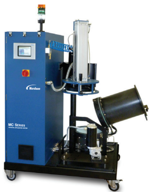
Tiltable tank for easy cleaning and maintenance
