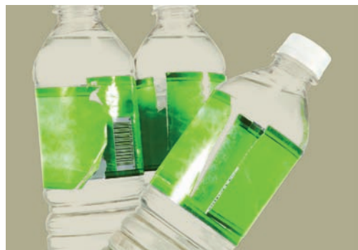
Misapplied, skewed labels and continual cleaning are common with wheel-pot labeling systems
