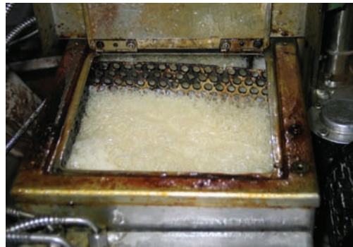
Open systems expose adhesive to contaminants and faster degradation
